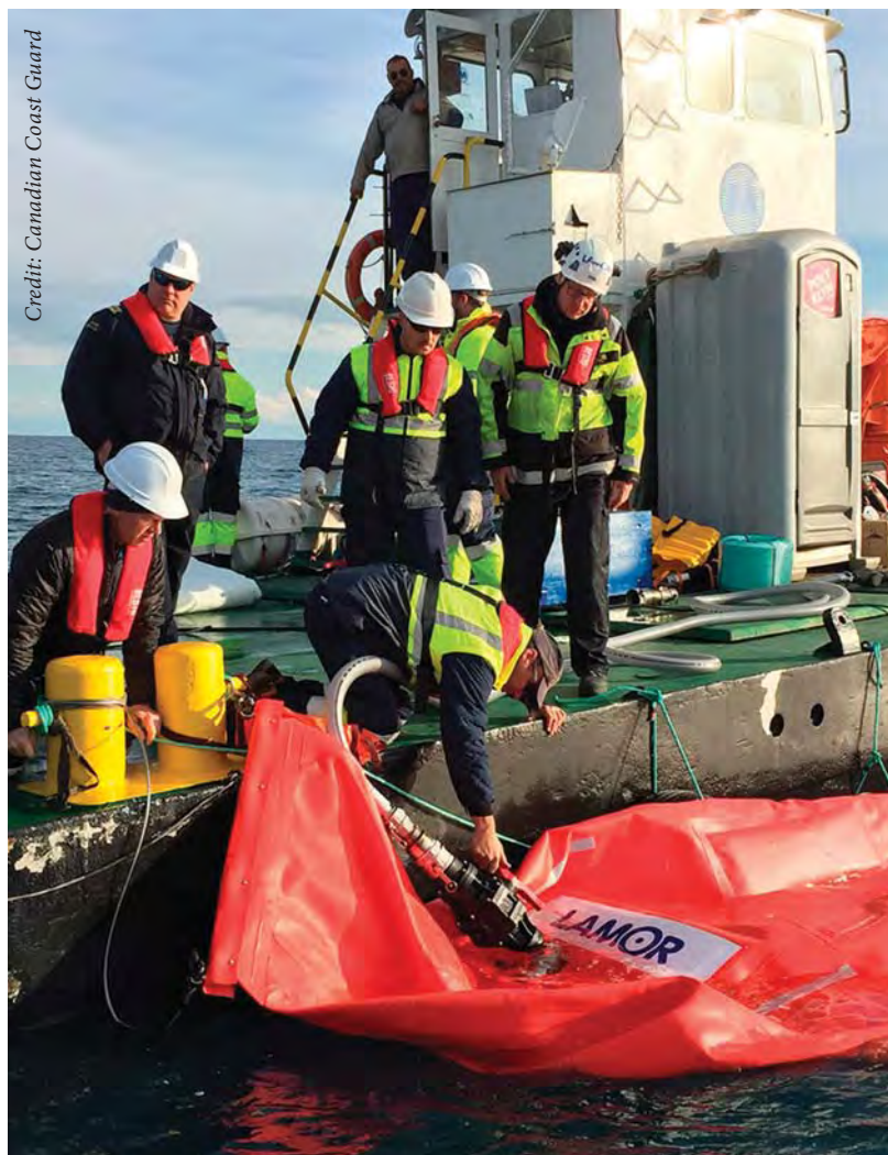
Canadian Coast Guard crews operate a towable floating bladder for storing recovered oil.
