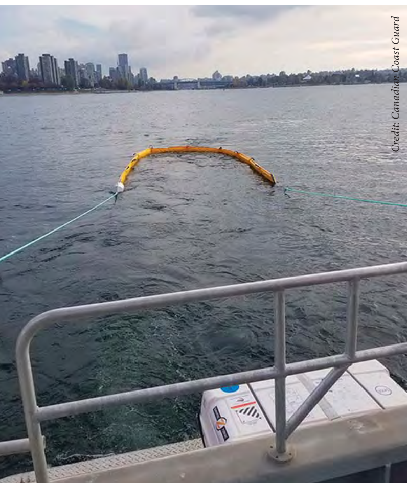
A fence boom for containing pollutants is employed in this undated photo off Vancouver, BC.
