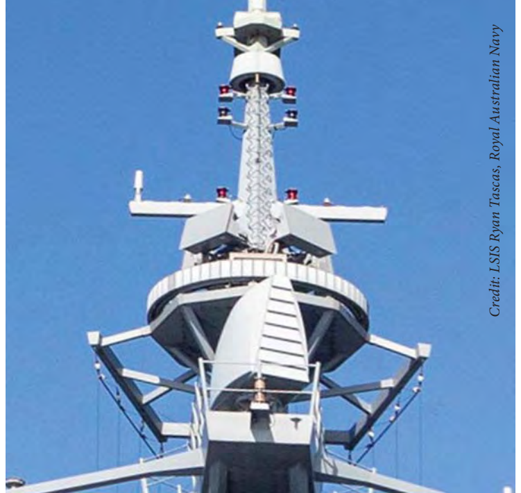
The AN/USG-2 antenna used to transmit data as part of the Cooperative Engagement Capability can be seen in this 9 March 2021 photo of HMAS Hobart's mast, taken during Exercise Tasman Shield 21 off Australia's east coast. The antennas are the two rectangular planar arrays in the centre (two more arrays face aft to ensure 360 degree coverage).
