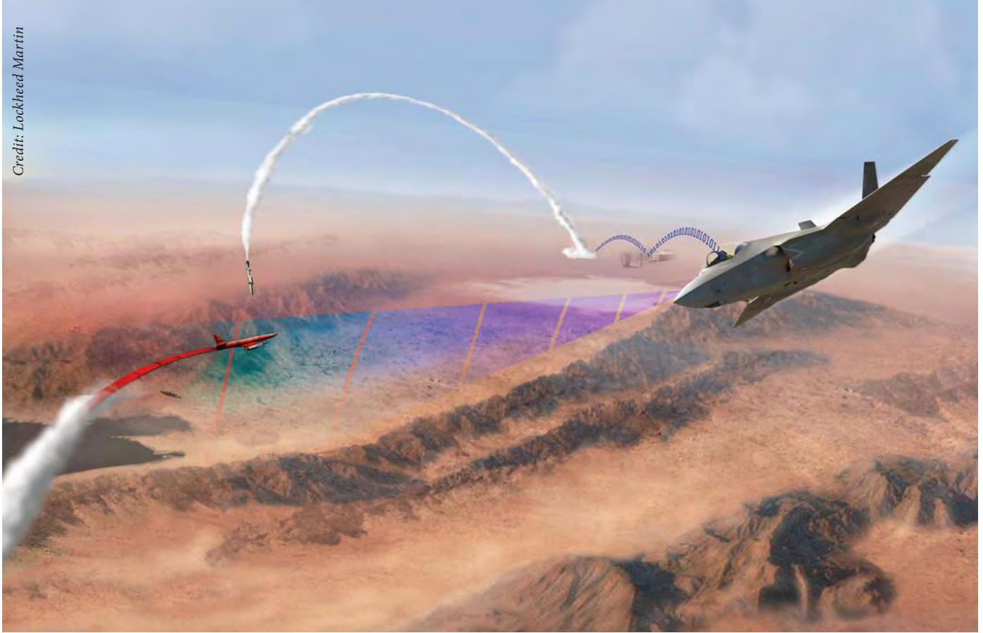
A graphic illustrating a 2016 test of Naval Integrated Fire Control - Counter Air (NIFC-CA), whereby an F-35B Joint Strike Fighter sent targeting data to a land-based SM-6 Standard Missile launcher to maximize the missile's range. CEC is an enabler of NIFC-CA
