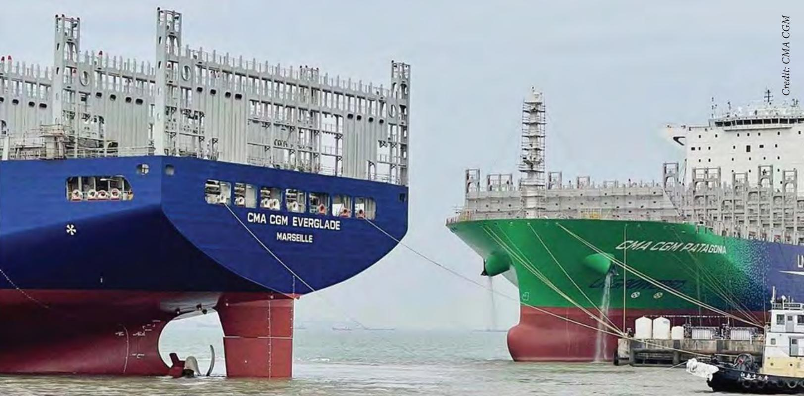
Two LNG-powered container ships of the French shipping line CMA CGM are pictured here during trials in China in July 2021. Note the single propeller arrangement, which may reduce manoeuvrability at low speeds, increasing the risk of situations like that experienced by *Ever Given*.
