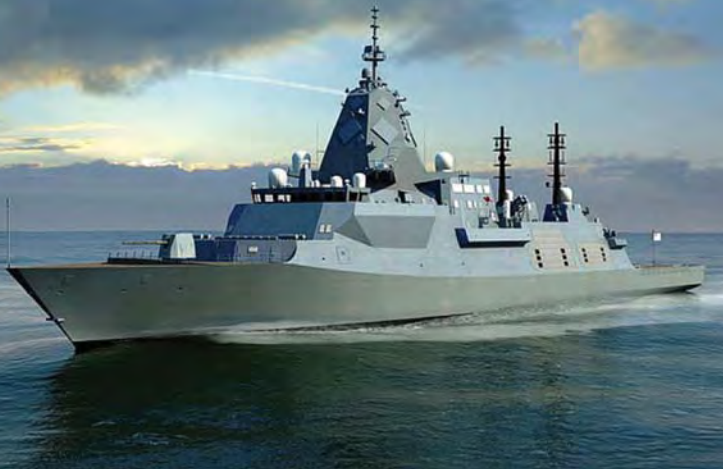
A computer-generated graphic of the Australian navy's future Hunter-class frigate. The Hunter-class will use the same Type 26 hull as the Canadian Surface Combatant but with major changes to incorporate the Australian CEFAR2 radar suite and Saab Australia combat system.
