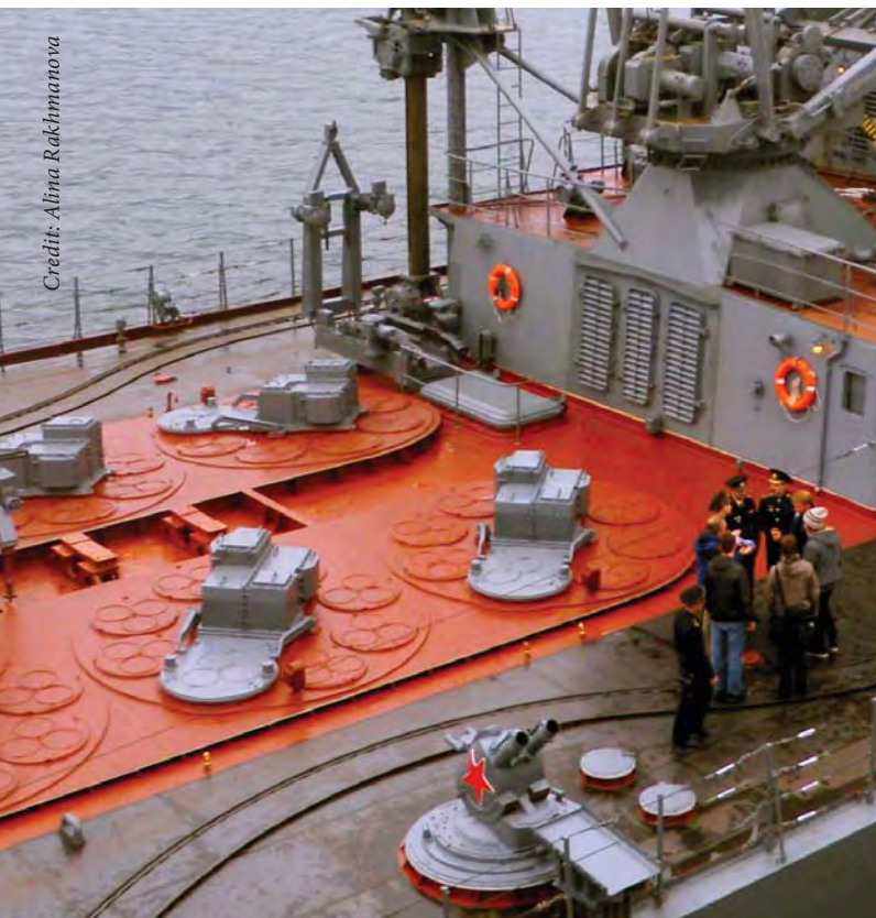
A close-up of the long-range SA-N-6 surface-to-air missile cells on RFS Varyag , sister ship to Moskva , during a port visit to Vancouver, BC, in November 2012. The seeming failure of Moskva to employ any of its anti-air defence systems throws into question the efficacy of the defence suites of other Russian warships.
