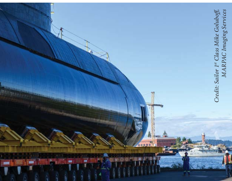
The Victoria -class submarine HMCS Corner Brook begins the undocking process following its Extended Docking Work Period at Esquimalt, BC, in June 2021.
