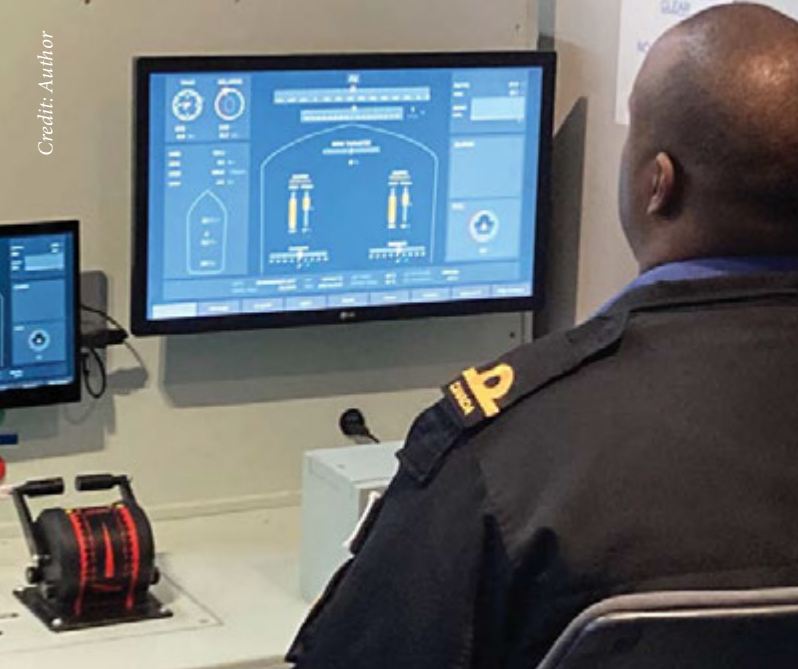
An RCN sailor operates the helm console of the bridge simulator. The console was built from scratch using MDF boards based on dimensions of those for the Orca-class training craft.
