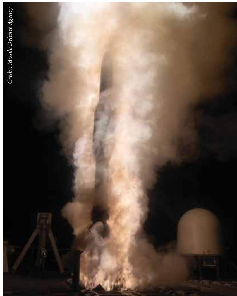
A SM-6 Dual II missile is launched from USS Preble's Mk 41 Vertical Launch System near Hawaii during a flight test on 28 March 2024. The test resulted in the successful interception of a medium-range ballistic missile.
