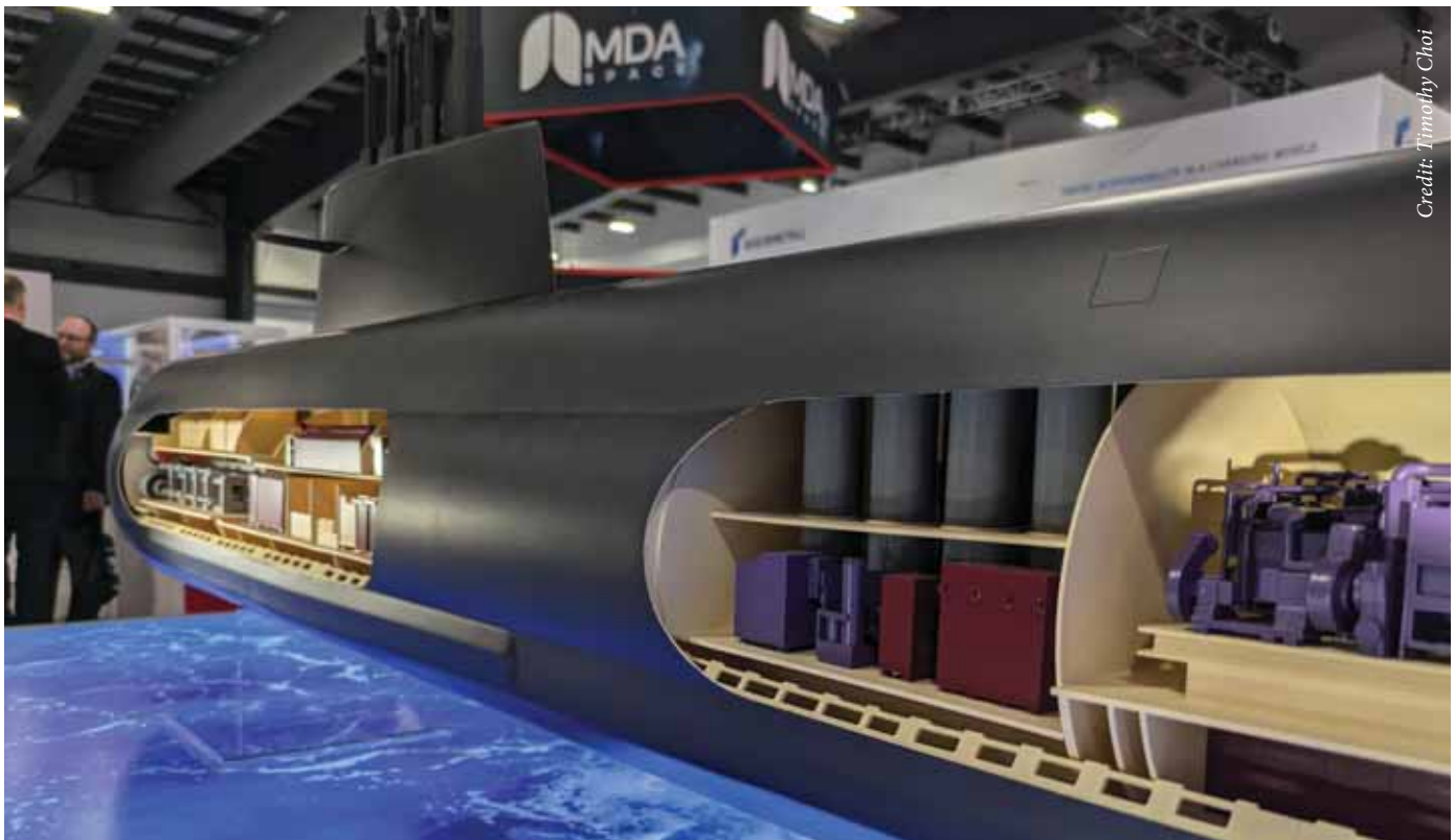
A model of the Korean KSS-III diesel-electric submarine, with a cutaway showing its large-diameter ballistic missile launch tubes. The KSS-III is one of the likely contenders for the Canadian Patrol Submarine Project. This model was on display at the Hanwha booth at the CANSEC 2024 tradeshow in Ottawa, May 2024.
